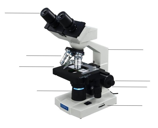
arm - course focus - eyepiece - fine focus - lamp control - light - objectives - stage
